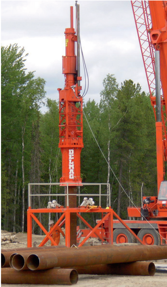
Diesel pile hammer D30-32 with rope suspended lead MAR 30-30
